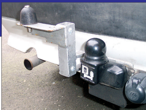
● Fig. 3: The tow ball was then re-fitted permanently. When G3UCA wishes to use the bracket, it slots over the protruding bolts, and is retained with two star washers and two additional nuts (see text). The G3UCA mobile whips are mounted onto the left hand side of the bracket using a 'gum boil' style mount (top left). It provides a very stable mount and also a very good earth which is necessary for efficient mobile operation (see text).
